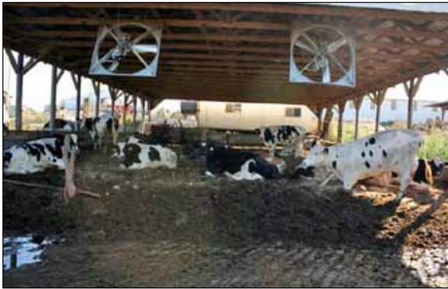
Figure 18. To minimize wetness, build multiple, narrow entrances along the long side of the barn. Entrances should be spaced every 50 feet.
