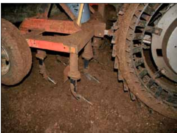
Figure 52. Most compost bedded packs are tilled twice daily with a field cultivator. Many different types of tillage implements have been used successfully.
