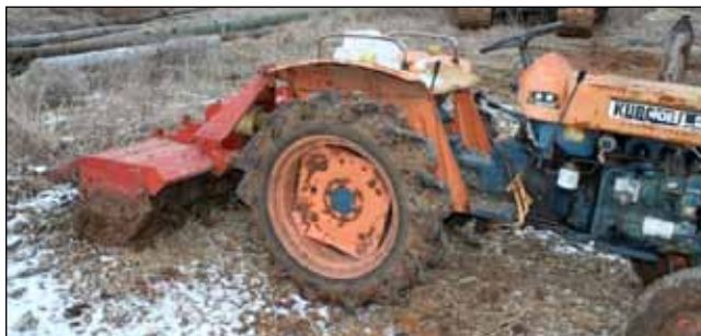
Figure 54. Roto-tillers are helpful to break up clumps of bedding material and maximize oxygen/air infiltration.
