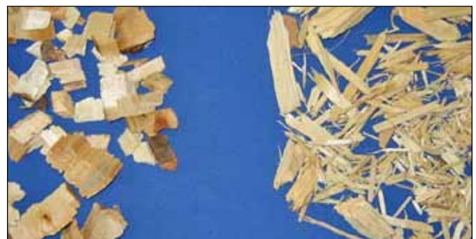
Figure 58. Wood chips produced with sharp blades (left) and blunt hammer (right).
