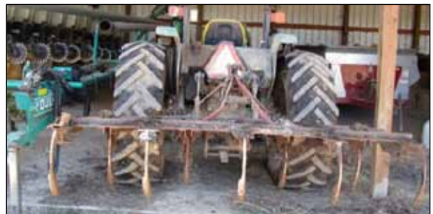
Figure 54. Roto-tillers are helpful to break up clumps of bedding material and maximize oxygen/air infiltration.
