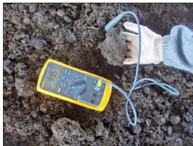
B. Example of compost that is too wet with insufficient temperature.
