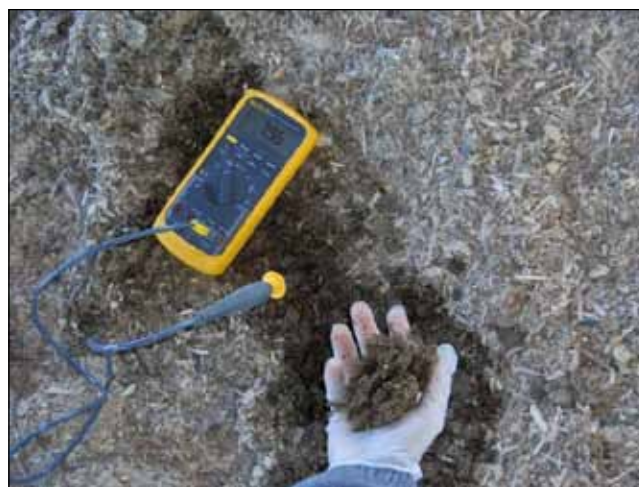
C. Example of compost that is too dry with insufficient temperature.
