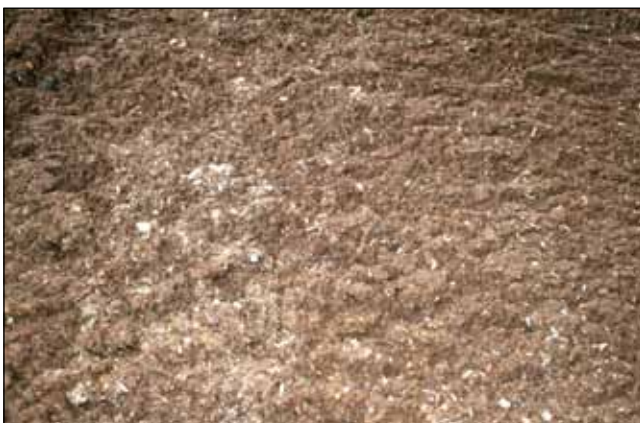
Figure 44. These pictures are examples of properly functioning composting processes. The material is dry and fluffy.
