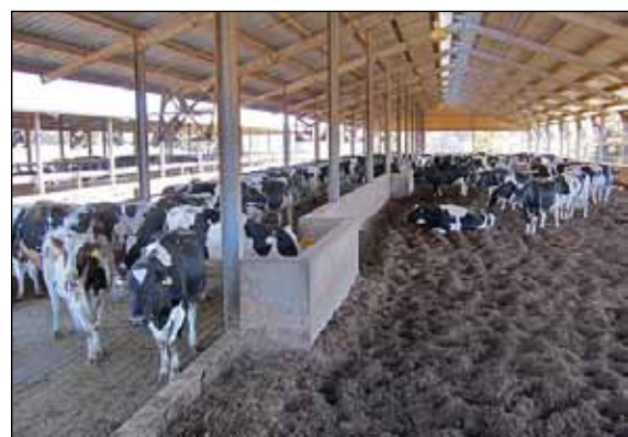
Figure 7. Recommended layout with feed alley, feedbunk, waterers, retaining walls, walkways, and open resting area.
