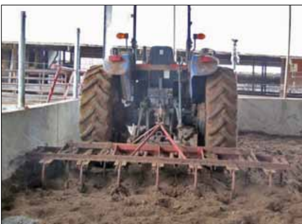
Figure 52. Most compost bedded packs are tilled twice daily with a field cultivator. Many different types of tillage implements have been used successfully.
