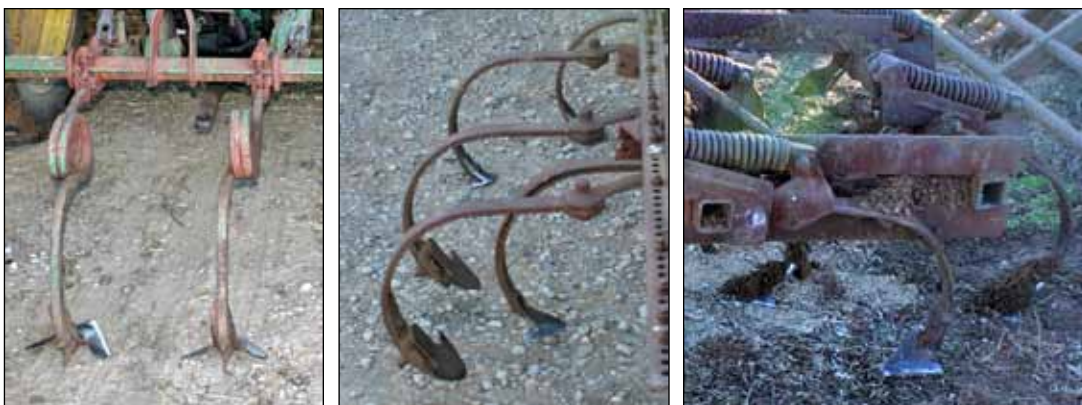
Figure 53. Sweeps or shovels may be added to tillage implement tines to provide more effective stirring. This is a cheap, effective addition to existing implements.
